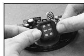
Put the new antenna on its header and fix it with the clamp.
