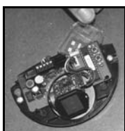
Remove the narrow sensing field antenna from its location.
